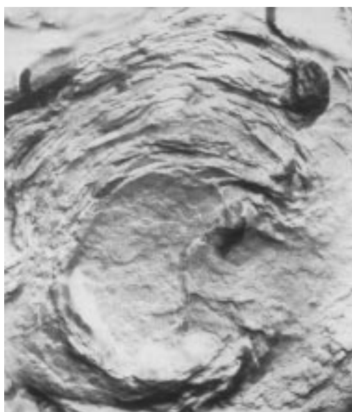
Fig. 4 Electron microscope image of freeze-fracture of liquid crystalline layers in an emulsion (reproduced with permission from ref. 9)
